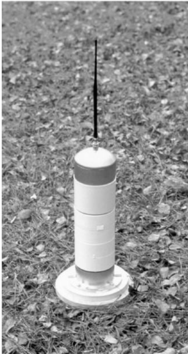
Figure 9. Seismic telemetry transmitter. Weather-proof PVC housing.
